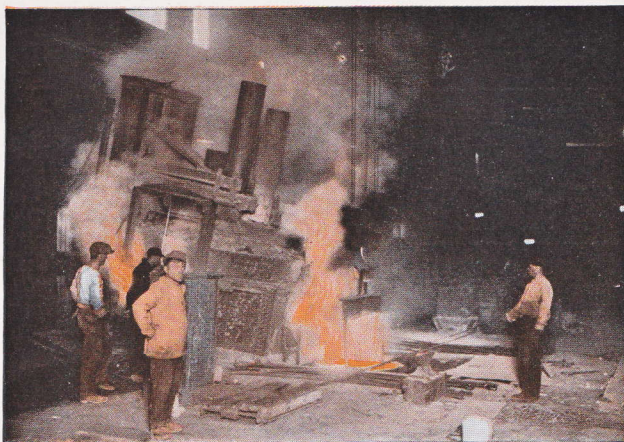
Six ton Cold Melt Electric Furnace pouring into six ton capacity ladle
